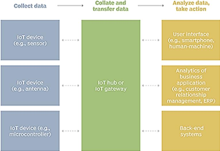
An example of how an IoT system works from collecting data to taking action.
